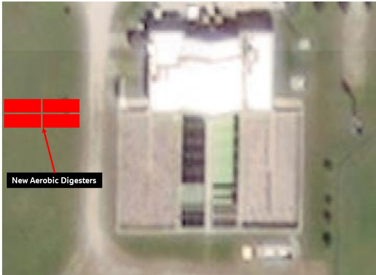
Figure 8-3. Plympton WWTP Aerobic Digester Upgrades - Footprint Required
