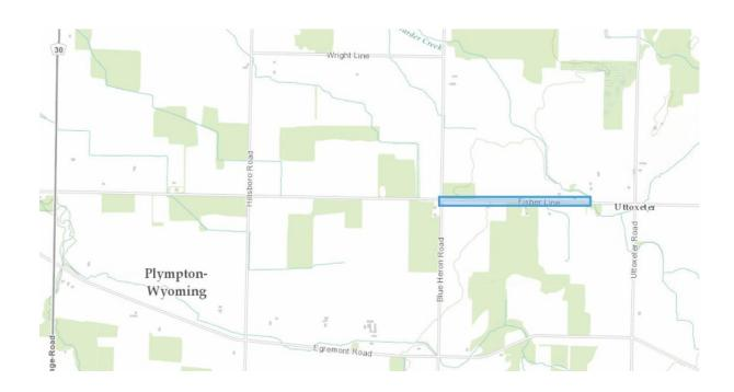
The proposed works for the 2025 construction season will consist of pulverizing the existing surface treatment, the addition of sub-drains, minor ditch re-grading, placement of additional granular road base and hard resurfacing.
