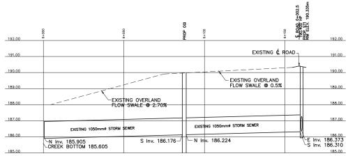
EXIST 87.5m OF 1050mmø STORM SEWER @ 0.31% CONCRETE PIPE | CSA A257.2 65-D EXIST 73.0m OF 1050mmø STORM SEWER @ 0.12% — CONCRETE PIPE CSA A257.2 65-D
